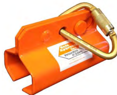
Model 00620 – Rail Grabber Fits 40lb/yd to 115lb/yd track 5,000lb Anchorage Point
