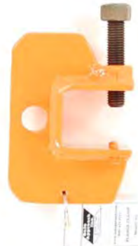
Model 00699 – Flange Clamp Great for attaching to a C-channel or other single flange anchor point. Fits 1/2" - 2-1/4" flange thicknesses 5,000lb Anchorage Point
