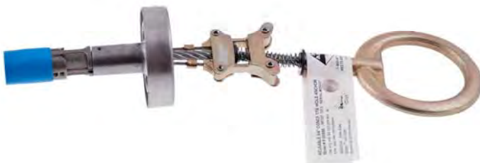
Model 00655 – Hole Anchor Fits 3/4" diameter concrete hole Easy release button 5,000lb Anchorage Point
